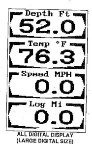
The large digital selection erases the chart and shows the digital displays in large numbers. Pressing the menu key gives only one menu page which is different from other menus. This menu lets you go back to chart information, placing the digital display back in the medium size. It also lets you select digital displays and adjust the depth alarm. Returning to the chart restores the normal menu operation.
